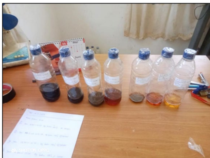
Figure 1. Solar oil, kerosene, and petrol from pyrolysis of LDPE plastic waste
